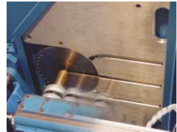
Trackplate works like a railroad switchyard.
